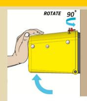
With bait in place, guide the top box back to its closed position and rotate the red button 90 degrees to lock it.
