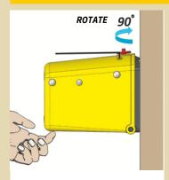
While supporting the top box with one hand, rotate the red button 90 degrees to unlock it.
