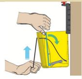
Once you feel it go over centre and start to release, slowly allow the setting cord to be drawn back into the trap, releasing the spring tension, and unsetting the trap.
