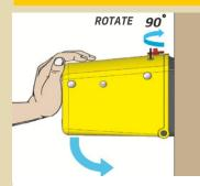
Support the top box with one hand and rotate the red button 90 degrees to unlock it. With the top box now free to pivot, guide it downward until it comes to rest on the tree or post.
