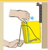
Gently push the back of the protruding bait bar forward, while keeping tension down on the setting cord.
