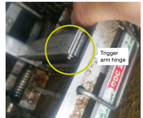
Figure 6. Aerial view of hinge connecting trigger arm to trigger hanger.
